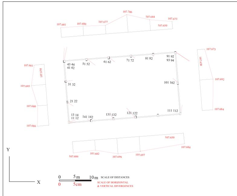
Fig.2 Horizontal and vertical divergences of the columns of the two floor precast construction.
