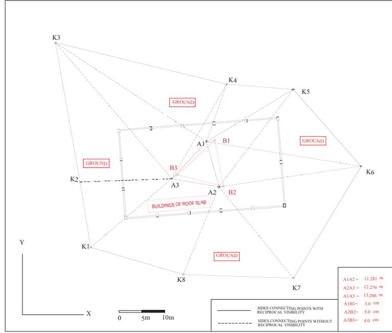
Figure 3. The control network for the determination of the horizontal movement of the building's roof slab.
