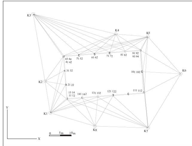
Fig. 1. The established geodetic control network for the detection of the divergences of a two-floor precast concrete building.
