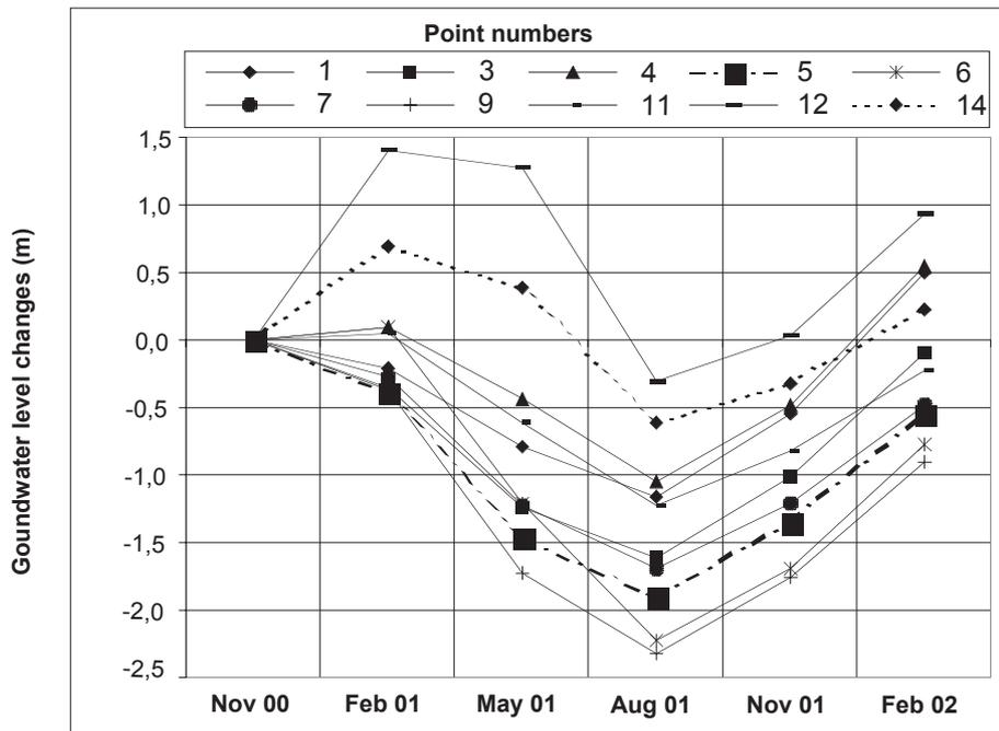
Figure 4. Groundwater levels changes at network points
