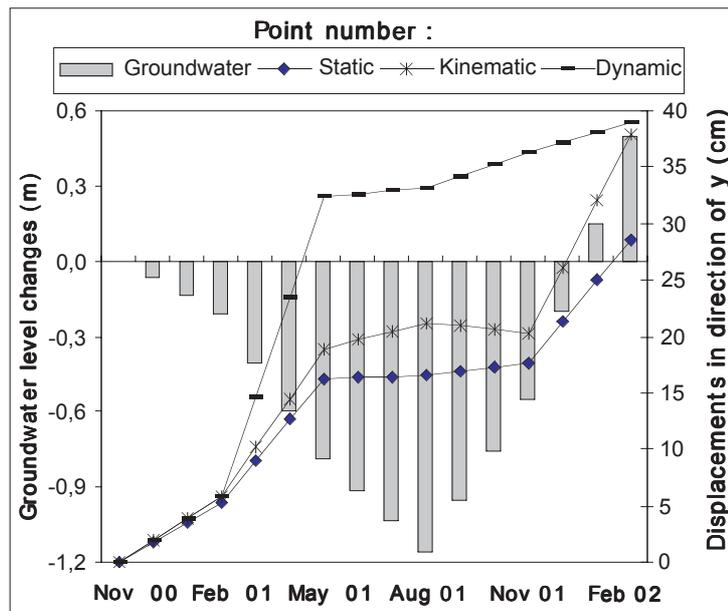
Figure 7. Relationship between static, kinematic, dynamic displacements and groundwater level changes
