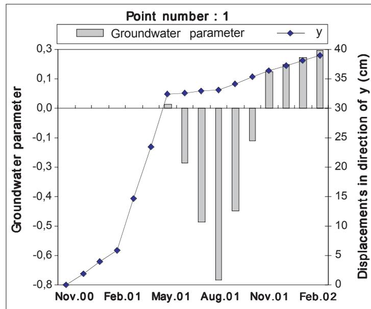
Figure 8. Relationship between acceleration effects of groundwater level changes and displacements
