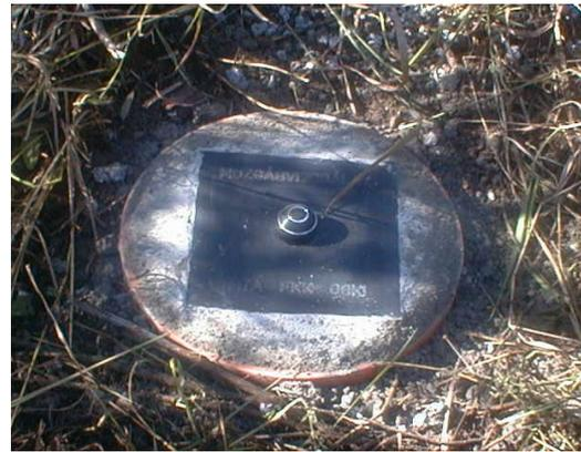
Fig. 3. Universal benchmark in borehole
