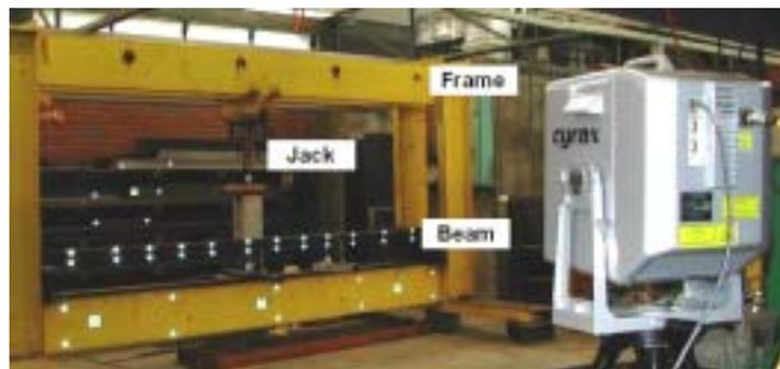
Fig. 1: Wooden beam, hydraulic jack system, reflective targets and the Cyrax 2500.
