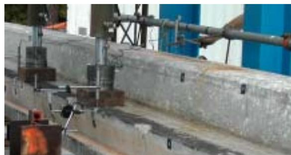
Fig. 4: Photogrammetric targets co-located with dial gauges and LVDTs.
