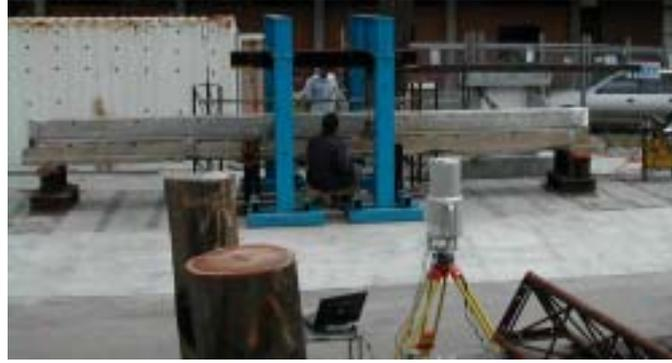
Fig. 3: Concrete beam (in the load testing frame) and the I-SiTE R-350 instrument.
