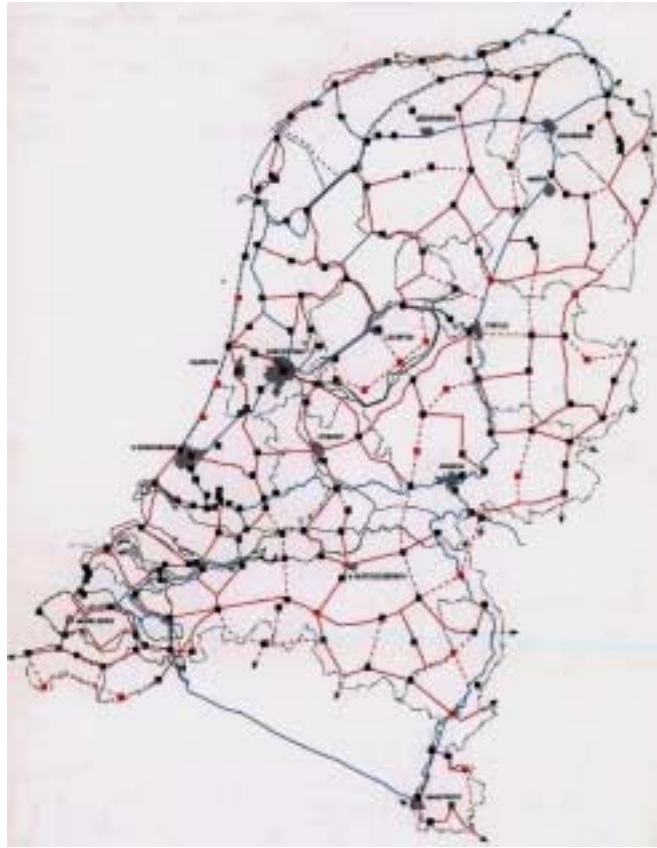
Figure 1: 5 th first order levelling network.
