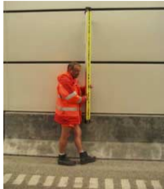
Figure No. 5 Levelling in Tunnel using invar-rod.
