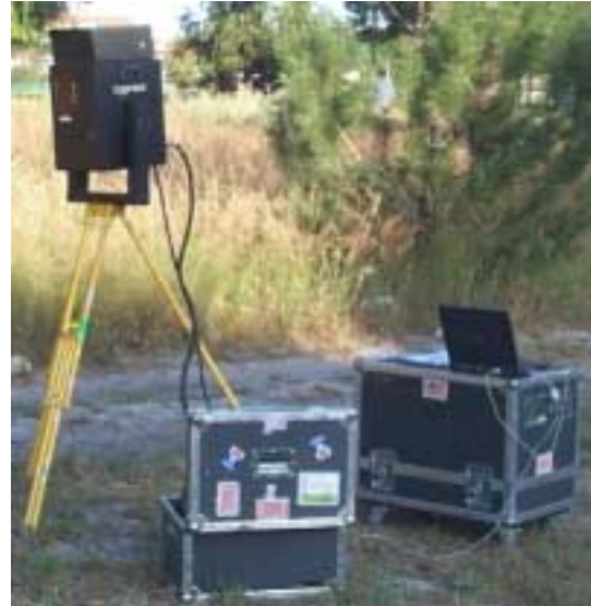
Figure 2: Cyrax 2400 Laser Scanner.
