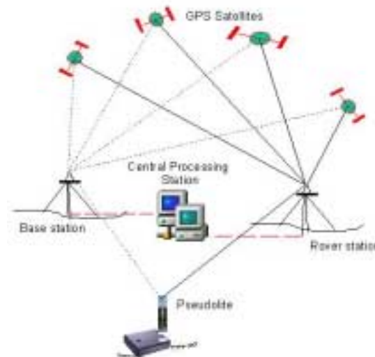
Figure 1. Configuration of a GPS deformation monitoring system augmented by pseudolite(s).
