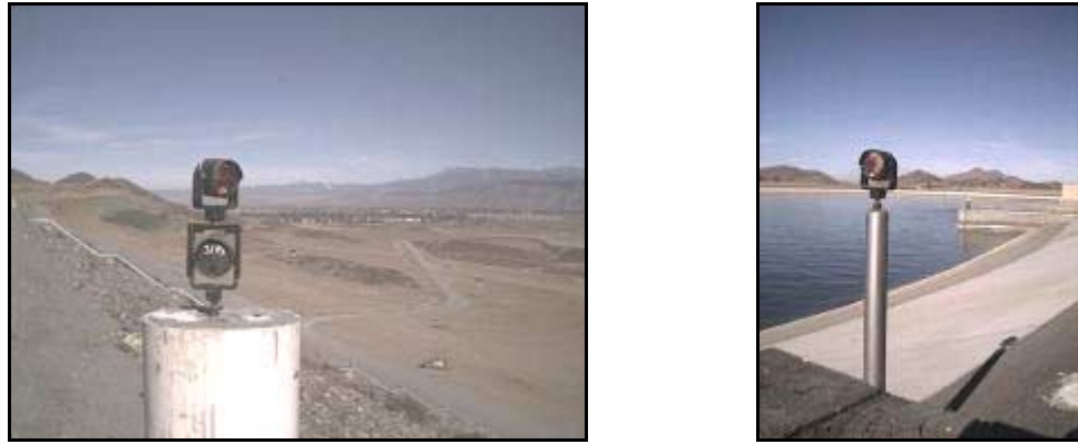
Figure 4. Pillar monuments with the target prisms.
