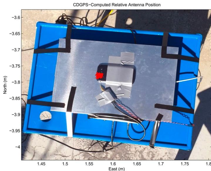
**Figure 4.4:** Result of carrier-phase GNSS solution using data collected from the antenna of a smartphone. The cluster of red near the lower left-hand corner of the phone represents 500 solutions over an 8-minute interval, superimposed on the photo and properly scaled [64].
