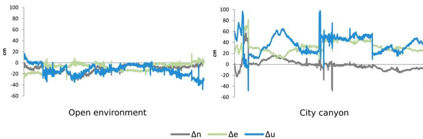
**Figure 7.3:** CSRS-PPP track deviations from the relative solution [129]
