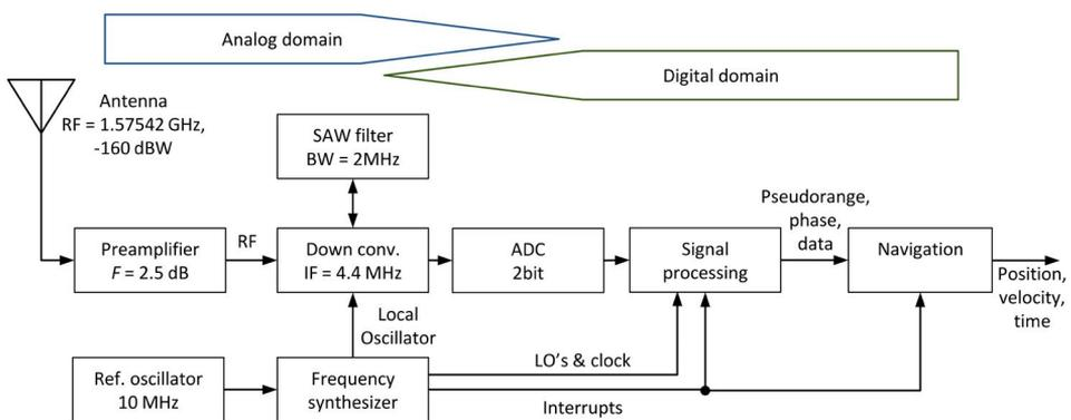
**Figure 4.1:** Example of building blocks for a GPS C/A-code L1 receiver [8, p. 373].
