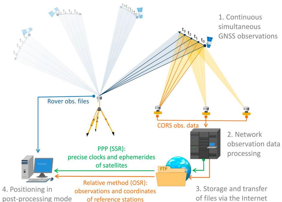
**Figure 3.4:** Post-processing using office software.
