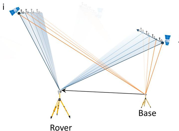
**Figure 3.1:** Relative positioning with phase double differences.
