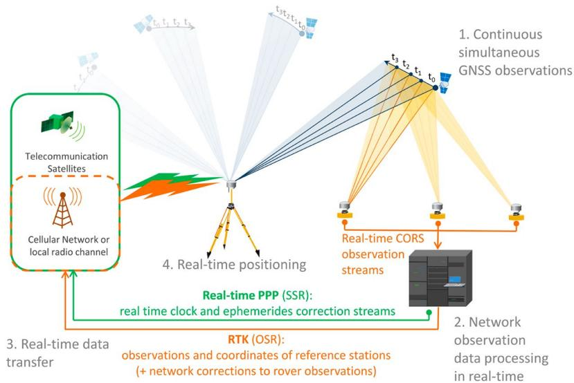
**Figure 3.5:** Real-time positioning scheme.
