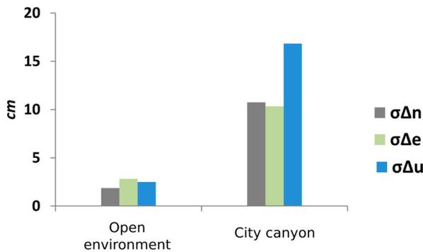
**Figure 7.4:** CSRS-PPP standard deviations from the relative solution [129]
