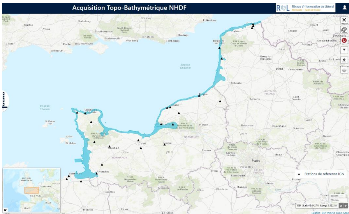
Figure 1: CORS distribution along survey area
