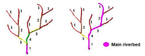
Figure 9. Example of calculating the main riverbed using the Shreve method.
