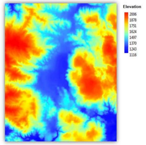
*Figure 4. Digital terrain-type elevation model generated by classification of altimetry points in the area of Tixtla, Guerrero.*
