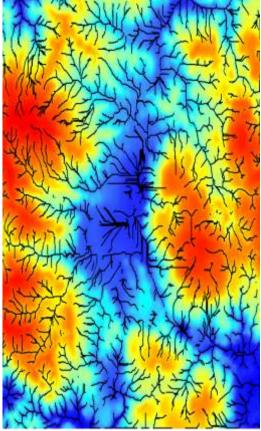
Digital terrain model and derived riverbeds with a flow accumulation parameter of 200 cells resulting in a network consisting of 3,937 segments.
