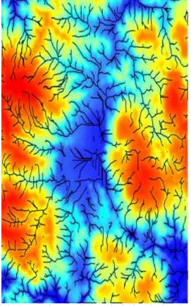
Digital terrain model and derived riverbeds with a flow accumulation parameter of 400 cells resulting in a network consisting of 1,919 segments.
