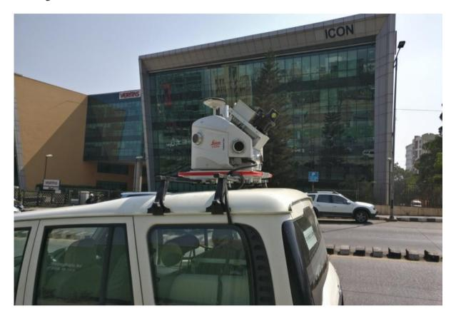
About 50 Km to 80 Km of city road network can be easily captured in a day using one unit of such mobile LiDAR system. Many solution providers are available in the industry viz, Trimble MX9, Leica Pegasus Two Ultimate, RIEGL VMX-2HA, Topcon IP-S3 HD1, Teledyne Optech's Maverick, HI-TARGET HiScan-C, with vide range of specification and price range to choose from.
