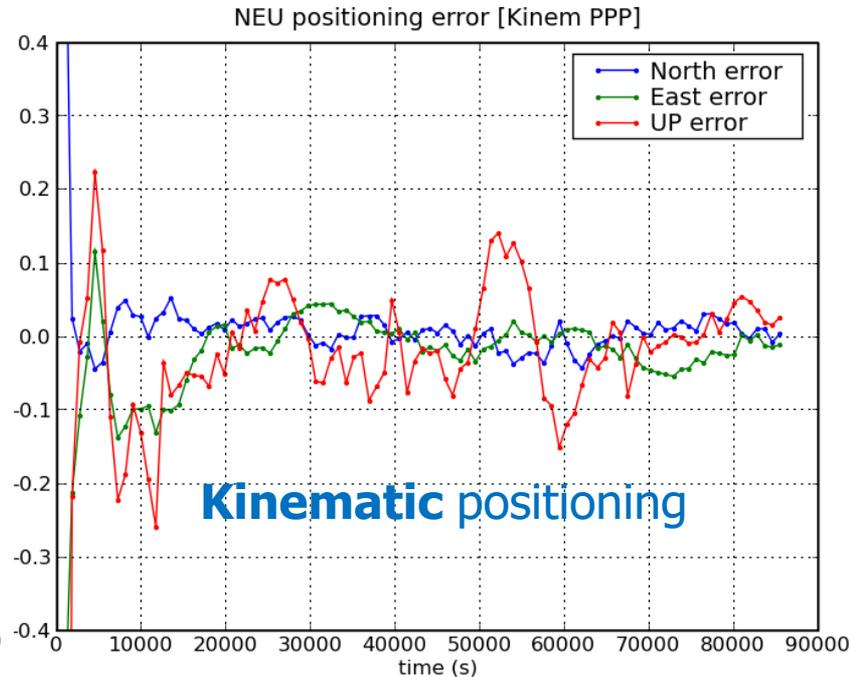
This high accuracy requires the use of code and **carrier measurements** and an accurate measurement modelling up to centimetre level or better.
