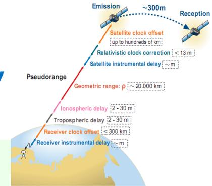
$$P_{Crec}^{sat} = \rho_{rec}^{sat} + c \cdot (dt_{rec} - dt^{sat}) + Trop_{rec}^{sat} + \mathcal{M}_{Pc} + \varepsilon_{Pc}$$
