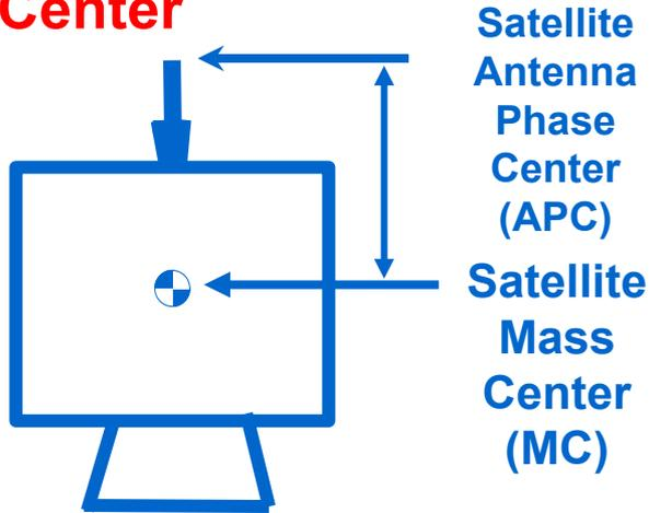
Broadcast orbits are referred to the antenna phase center, but IGS precise orbits are referred to the satellite mass center.
