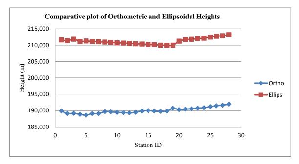
Figure 4: Orthometric and ellipsoidal heights pattern along the observed profile.
