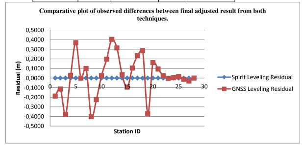
Figure 1: plot of residuals of adjusted spirit leveled heights and adjusted GNSS/Leveling heights
