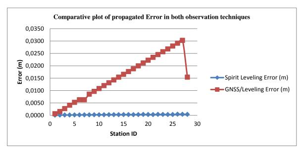
Figure 2: plot of values of standard deviation at stations from both techniques.
