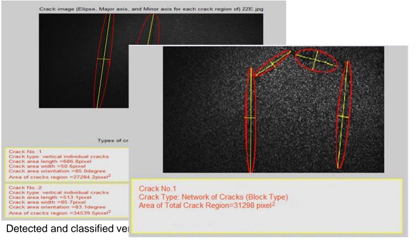
Detected and classified network of cracks (block type)
