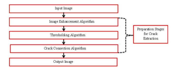
Focus on <u>local dynamic theshold algorithm</u> determinig window size and contrast value to take into account varying lightning conditions and shadows; more details in Al-Mistarehi & Schwieger (2015).
