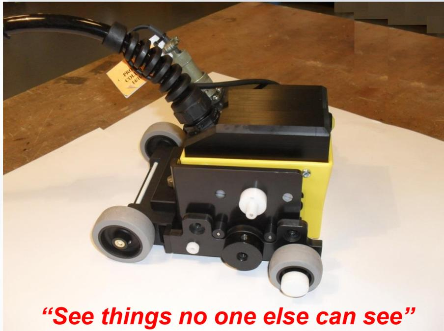
*Super High-Resolution antenna for concrete inspection*
