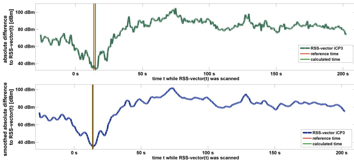
Figure 5: Euclidean distances of a certain iCP calculated from continuous RSS scans while walking along a trajectory
