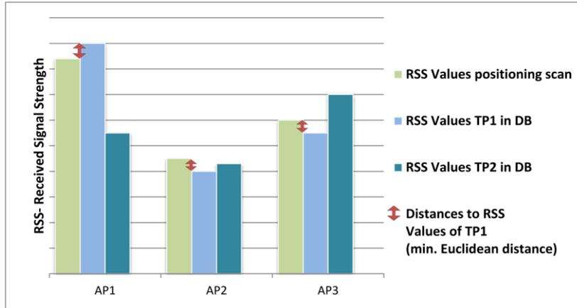
Figure 2: Allocation of positioning scans to training fingerprinting DB
