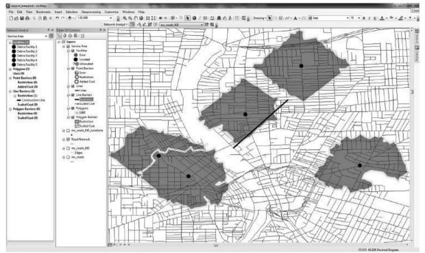
Figure (6) Debris cleanup service area network algorithm output results—areas 1000 meters from debris collection points (2014 ESRI, ArcGIS, ArcMap (Tomaszewski, 2015)).
