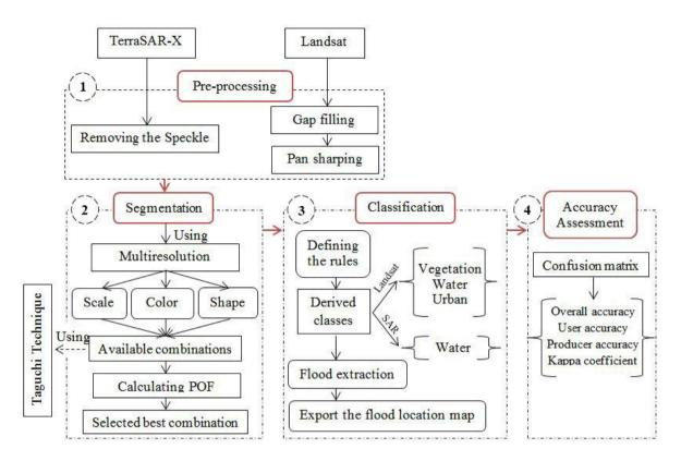
Figure 3: Overall methodological flow chart developed for the ensemble classification approach
