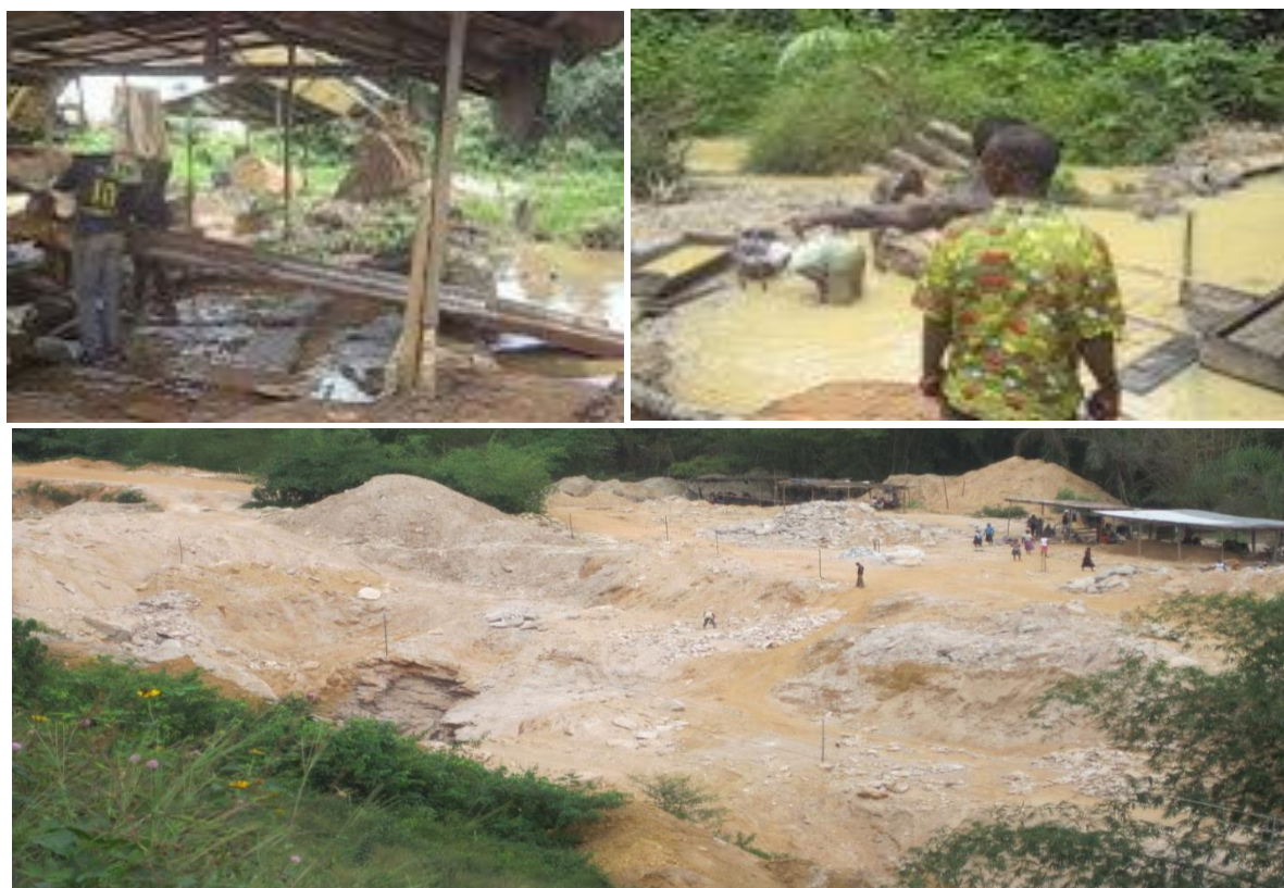
Fig. 1 Excavations, Grinding and Washing of Earth Materials for Gold at
