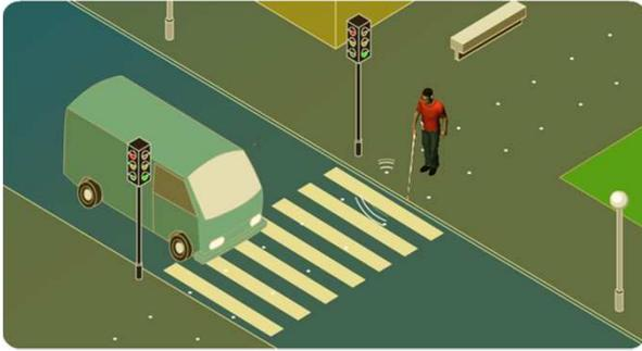
The idea consists in using **RFID** (Radio Frequency Identification) passive transponders (i.e. microchips) to create a path guiding a visually impaired person through a location. The walking stick has an embedded antenna (with a bluetooth transmitter) which detects/reads the RFID transponders.
