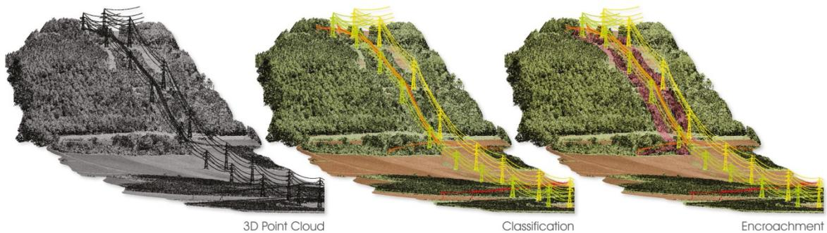
Fig. 11: Power Line Inspection
