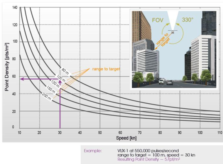
Fig. 4: Performance envelope-2, 550 kHz
