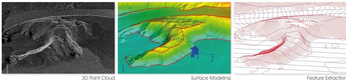
Fig.12: Surface Modeling, Feature Extraction
