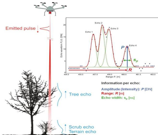
Fig.8: Interaction of Laser Pulse with Target
