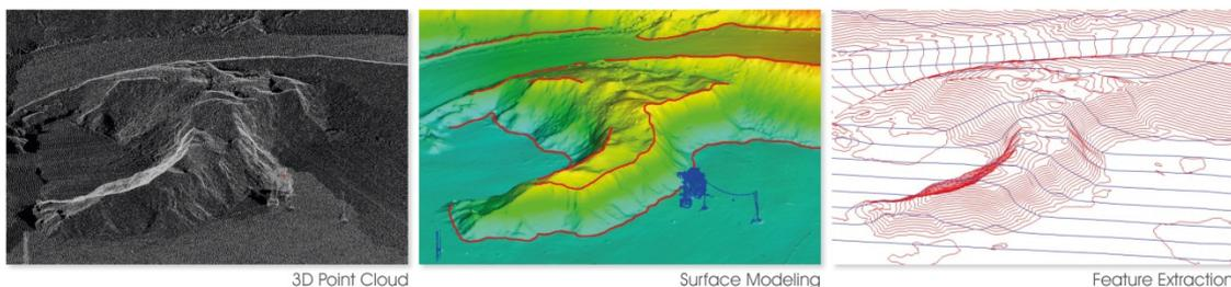
Fig.12: Surface Modeling, Feature Extraction
