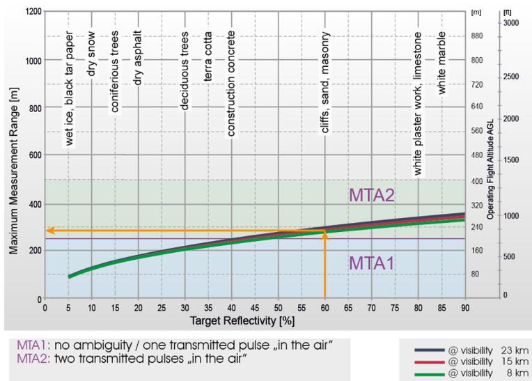
Fig.3: Performance envelope-1, 550 kHz
