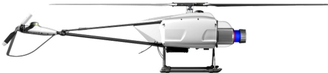
Fig.4: Example: planned integration of *RIEGL VUX-1* with Flying-Cam SARAH 3.0 ©
