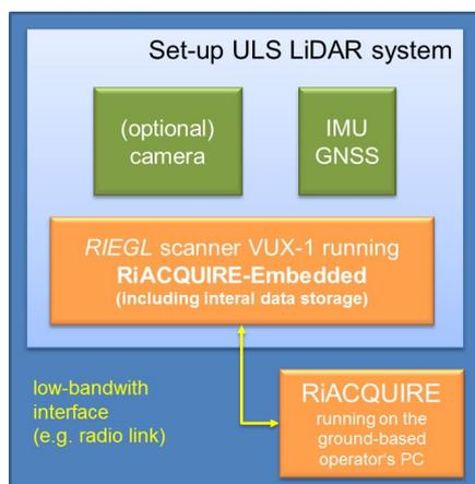
Fig.6: Set-up Unmanned Laser Scanner (ULS) LiDAR system
