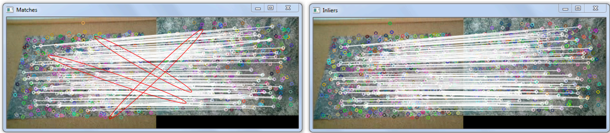
Figure 6. Matches between a random video frame and the pattern image before the rejection of the outliers by RANSAC (left) and inliers returned by RANSAC between the same random video frame and the pattern image (right).
