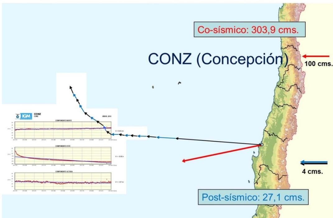
Fig 5. Post-seismic movement of CONZ station in Chile up to the year 2013.
