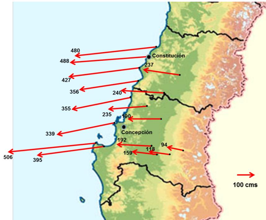
Fig 4: Coseismic movement with the Maule earthquake in 2010.
