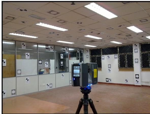
Figure 2: Self-calibration test field for the Faro Focus 3D scanner.
