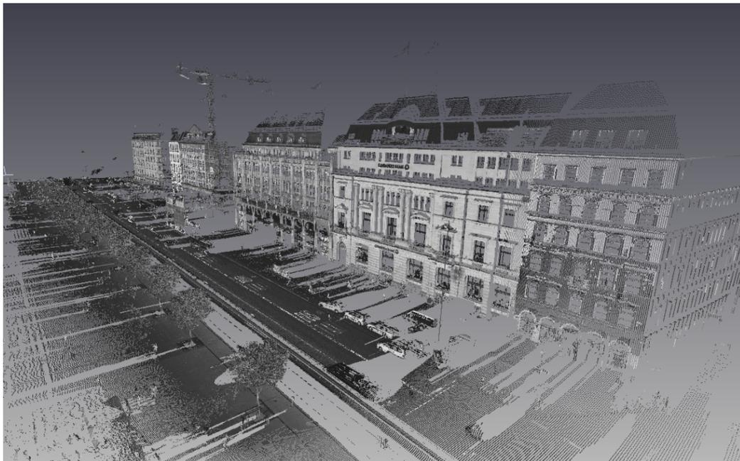
**Figure 8** Pointcloud from the mobile mapping system in Hamburg
