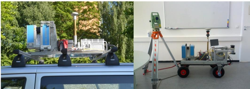
**Figure 2** Configuration of the system, left outdoor, right indoor
