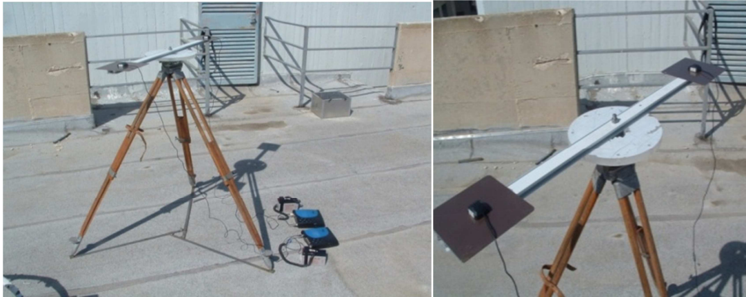
Figure 3: A direction finder constructed of two pieces: a pointer and a sensor.
