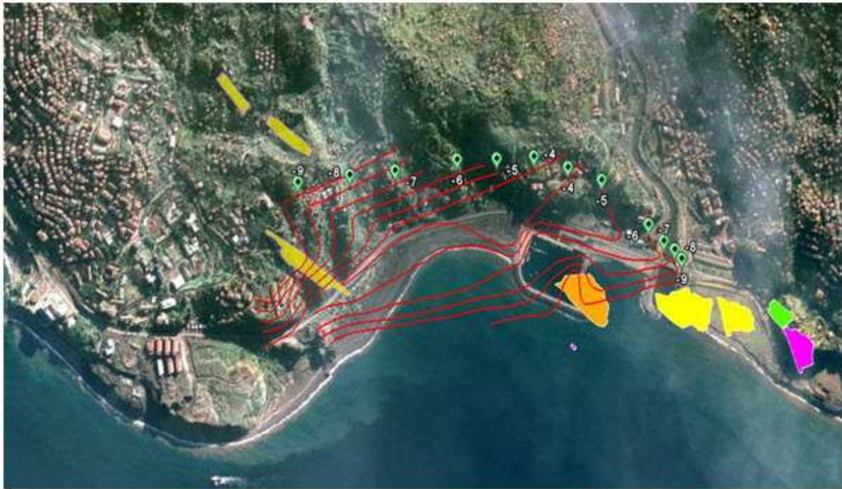
Figure 4. Subsidence counters from GNSS and leveling in period 2008-2010.
