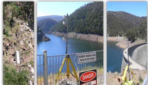
Figure 5b: LocataLite and receiver installation.
