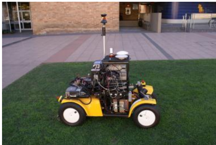
Figure 7: Integrated GPS+INS+Locata test car on UNSW campus.
