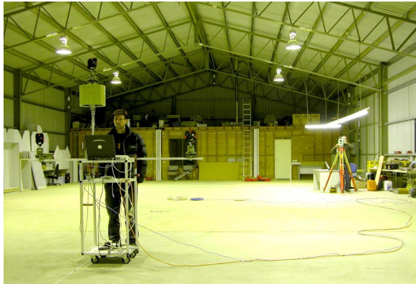
Figure 9: Indoor test site, Locata receiver on trolley and RTS setup.
