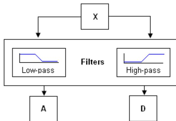
**Fig. 1.** The filtering process: the original signal X passes through two complementary filters and emerges as two signals (Approximation A and Detail D).
