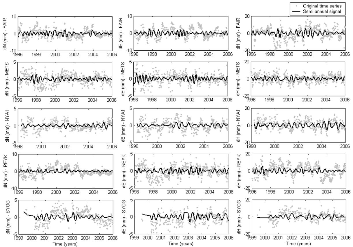
**Fig. 3.** Superposition of the original components (North, East and Vertical) of stations at high latitude with their semi annual signals (details 4) using discrete Meyer wavelet.
