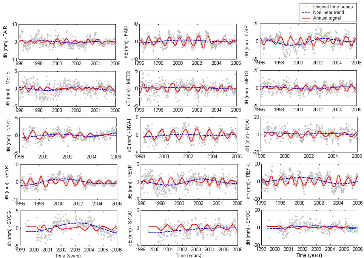
**Fig. 2.** Superposition of the original components (North, East and Vertical) of stations at high latitude with their nonlinear trend (Approximations 7) and annual signals (details 5) using discrete Meyer wavelet.
