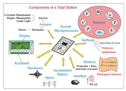
Fig. 3: Components of a modern total station
