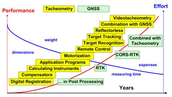
Fig. 2: The different steps of progress for tacheometry and GNSS during the last 20 years
