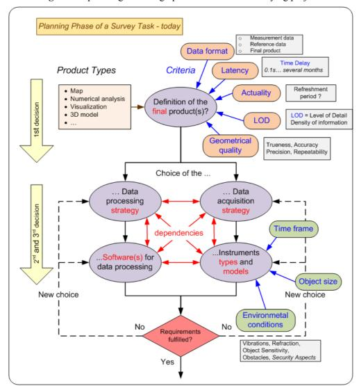
Fig. 7: The planning and design phase of an actual surveying project.
