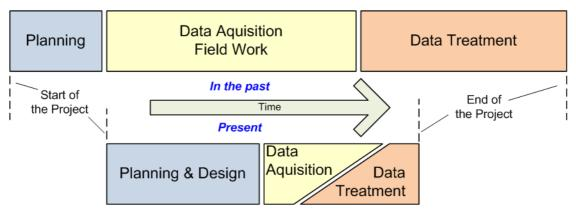
**Fig. 8b**: The different phases of a surveying project (not to scale).
