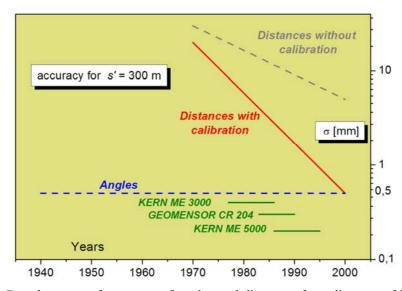
Fig. 5: Development of accuracy of angles and distances for a distance of 300 m.
