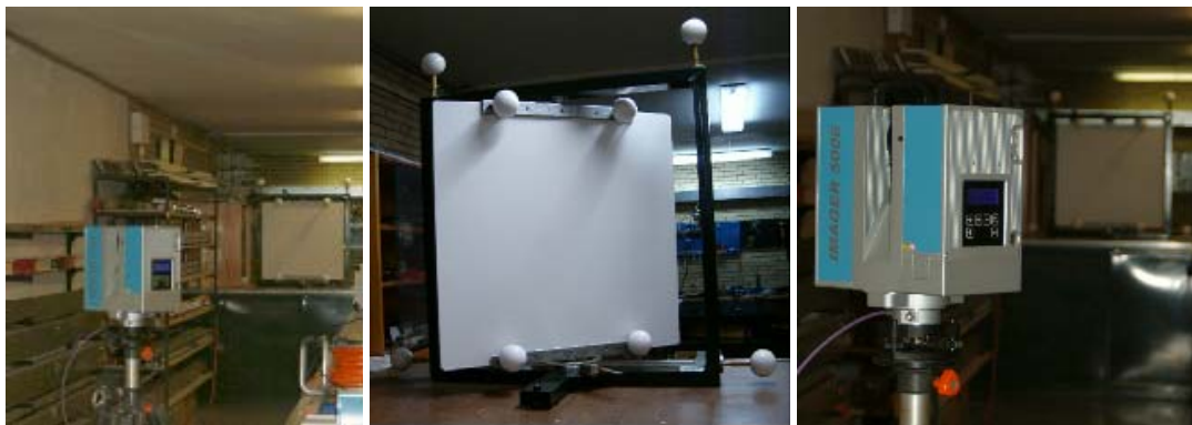
Figure 11: Scanning set up for the investigations into the laser beams angle of incidence on 3D accuracy with swivelling planar white stone slab (centre)
