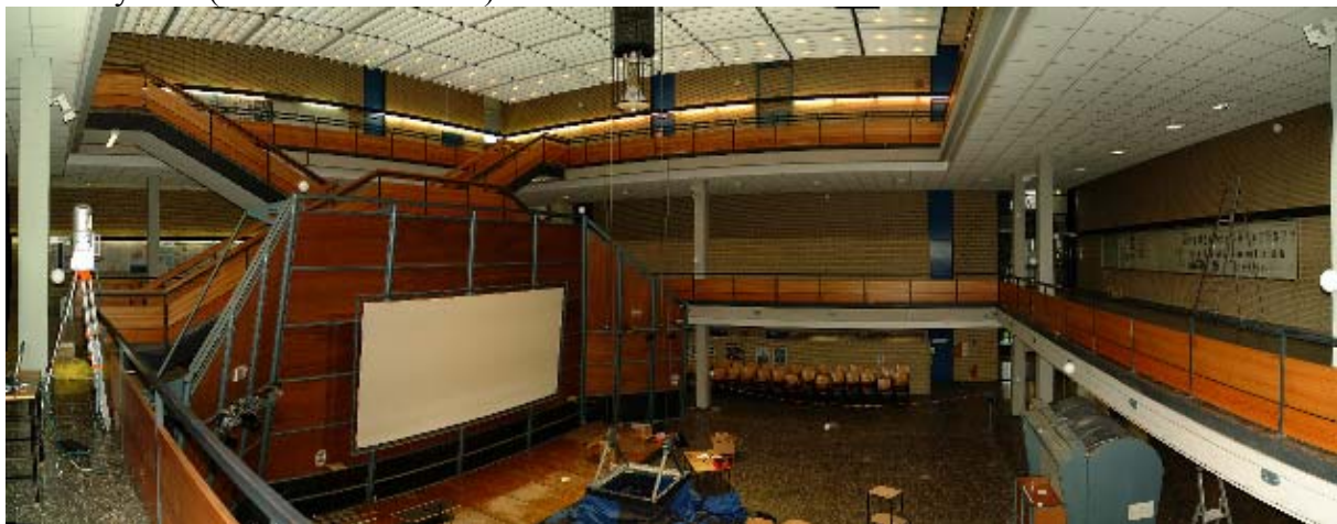
Figure 2: 3D test field at the HafenCity University Hamburg for geometrical investigations into TLS
