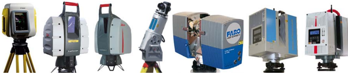
Figure 1: Terrestrial laser scanning systems for investigation at HafenCity University Hamburg: Trimble GX, Leica ScanStation 1 and 2, Riegl LMS-Z420i, Faro LS 880HE, IMAGER 5006 from Zoller & Fröhlich, and Leica HDS6000.
