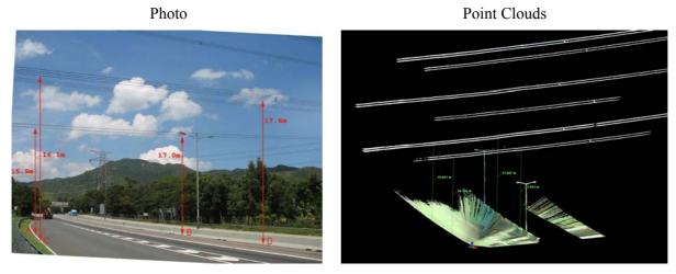
Figure 5 – Photo and Scanned Point Clouds of Overhanging Cables across Fanling Highway
