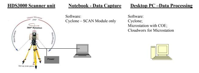
Figure 1 – Setup of Terrestrial Laser Scanning System
