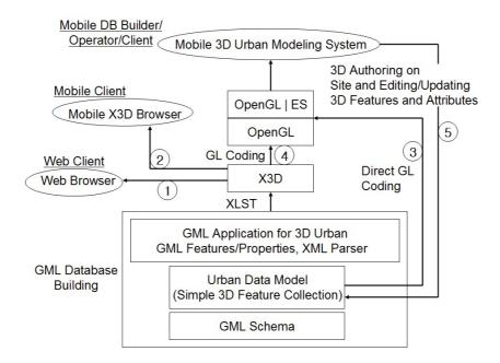
Fig. 8. Application strategy of mobile 3D and Web 3D for 3D urban visualization application.
