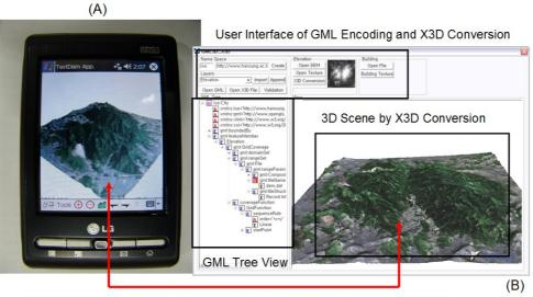
3D Terrain Model in Both Mobile 3D and Web 3D Graphics: Satellite Imagery superimposed on  $\mathsf{DEM}$
