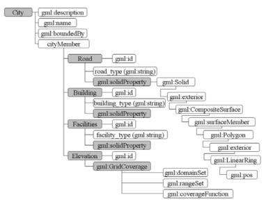
Fig. 3. GML application schema of urban modeling.
