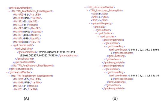
Fig. 4. GML encoding cases: (A) a part of the rail road in 2D, (B) a part of the subway structure in 3D.
