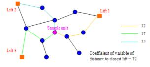
Fig.13. Example network analysis variable
