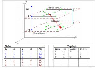
Fig. 10. 3D network data structure
