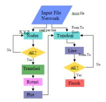
Fig. 11. Network visualization algorithm
