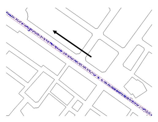
Figure 2. DGPS points distribution along the road segment under consideration in the EW direction
