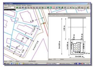
Fig. 7: Main window: The piping level is active Secondary window: Cross-section dimensioned
