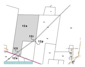
**Figure 9:** Servitude established for a pipeline. Parcel 11e, 11e and 11g is one real property, as well as 12a, 12l, 12o, 12p and 12r.
