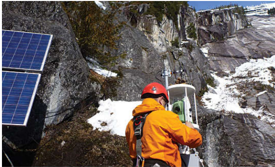
Figure 3. Total station in challenging monitoring conditions
