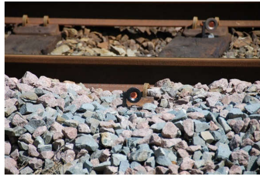
Figure 4. Picture of Prisms on railway from a total station
