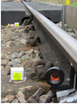
Figure 13. Prism and Tilt on the same Railway
