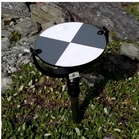
Figure 2: Tilt & Turn targets used in the 2015 UAV + TLS campaign.
