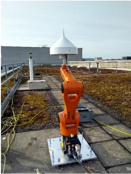
Figure 2: Robot arm with the GNSS antenna mounted. For the tests, the robot was moved back and forth with a 1D horizontal sinusoidal movement.
