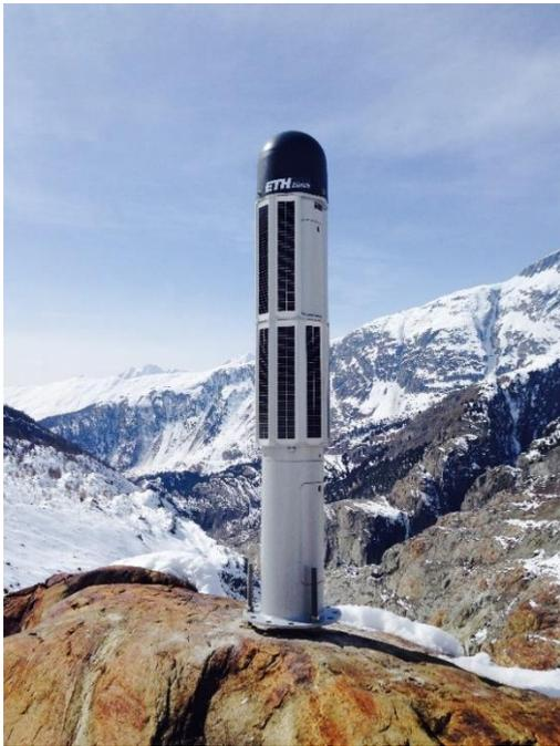
Figure 1: Example of a self-sufficient GNSS monitoring station, developed by the Institute of Geodesy and Photogrammetry of ETH Zurich (Image: Phillipe Limpach)
