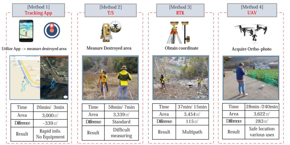
RTK is the most suitable method (Direct measurement method with rapid and good accuracy)
