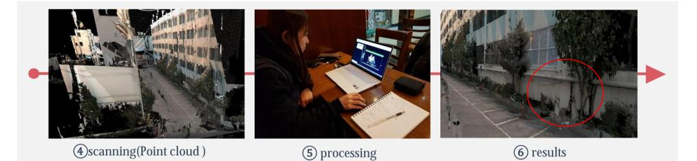
\*MMS(Mobile Mapping System) : rapid data acquisition method for 3D images with Camera, Laser scanner, GPS, INS, etc.
