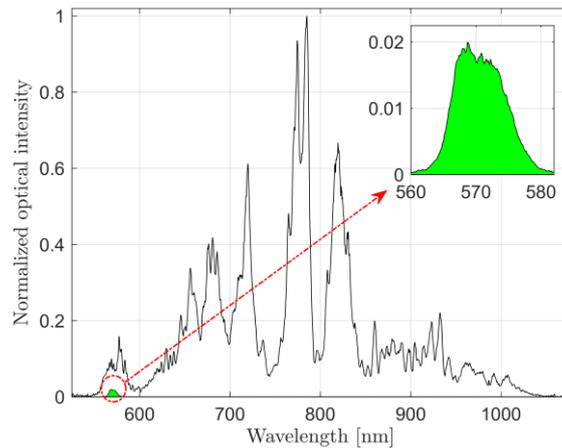
Fig. 2 Full supercontinuum spectrum of the applied laser setup, and filtered portion used for the measurements.
