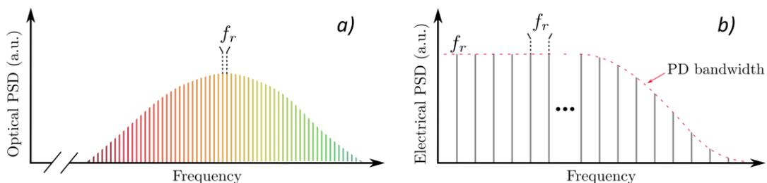
*Fig. 1 a) Optical frequency comb generated by a fs-laser with pulse repetition rate  $f_r$  (line density reduced for clarity, idealized power profile). b) Corresponding electrical frequency comb generated via intermode beating in the output of a photodetector (PD).*
