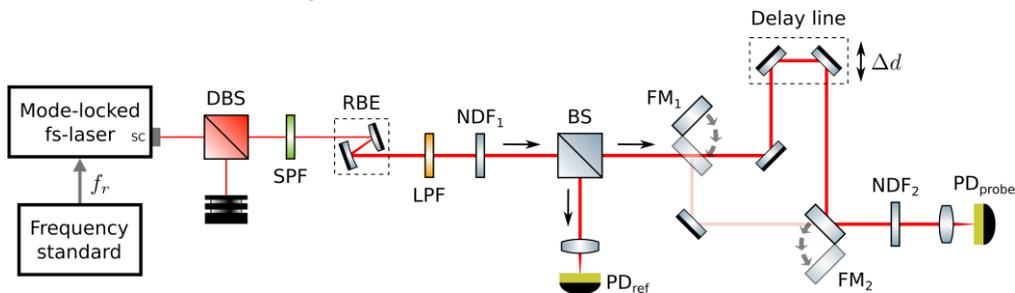
Fig. 3 Optical set-up for displacement measurements (DBS: dichroic beamsplitter, RBE: reflective beam-expander, SPF: short-pass filter, LPF: long-pass filter, NDF: neutral-density filter, BS: beamsplitter, FM: flip mirror, PD: photodiode)
