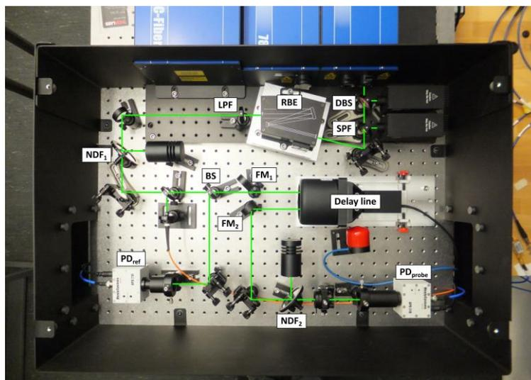
Fig. 4 Laser head (top) and optical set-up for displacement measurements.
