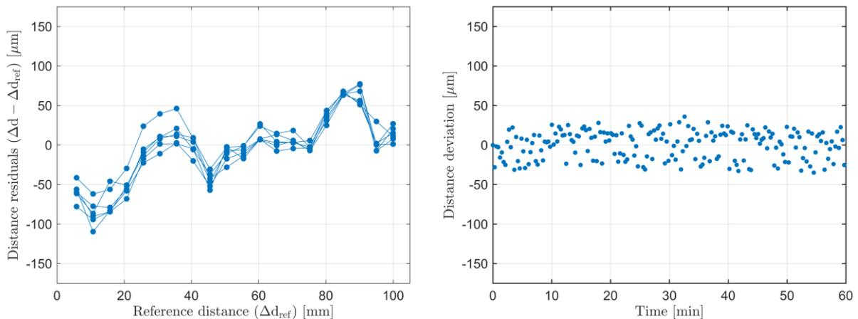
*Fig. 5 a) Distance residuals between measurements and reference values as a function of delay-line length. b) Deviations of static measurement as a function of time.*
