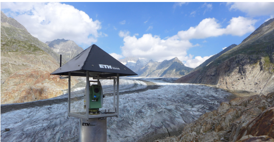
Fig. 4 TPS1 on its pillar with initial protective housing in place (picture: Geological Institute, ETH Zürich)
