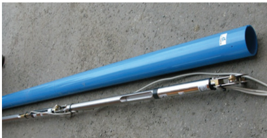
Fig. 6 In-place inclinometer and casing.
