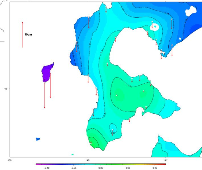
○ Vertical displacement model estimated from GEONET
