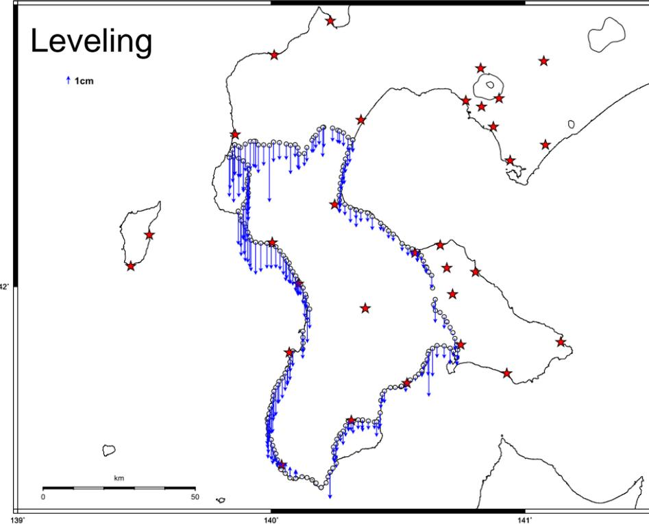
Vertical displacements on benchmarks from 2003-2004 to 2014 measured by leveling survey
