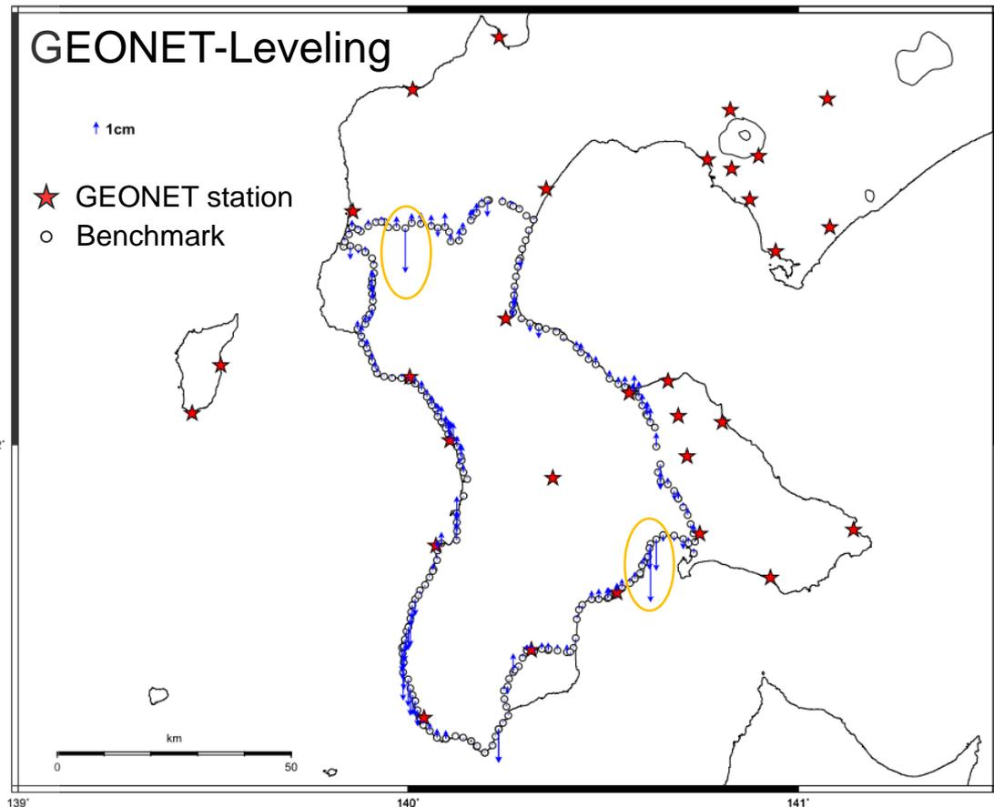
Difference between estimated displacement and leveling
