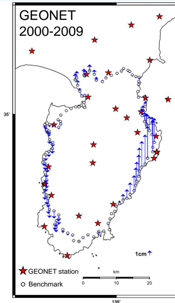
Vertical displacements on benchmarks from 2000 to 2009 estimated from GEONET
