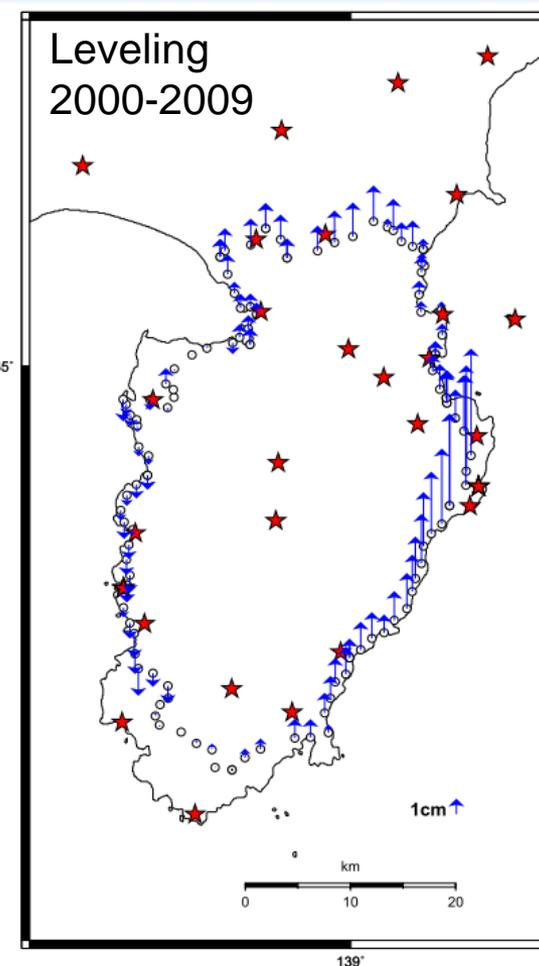
Vertical displacements on benchmarks from 2000 to 2009 measured by leveling
