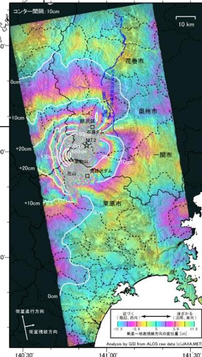
Coseismic displacements detected by InSAR image of ALOS caused by the Iwate-Miyagi Nairiku Earthquake in 2008.
