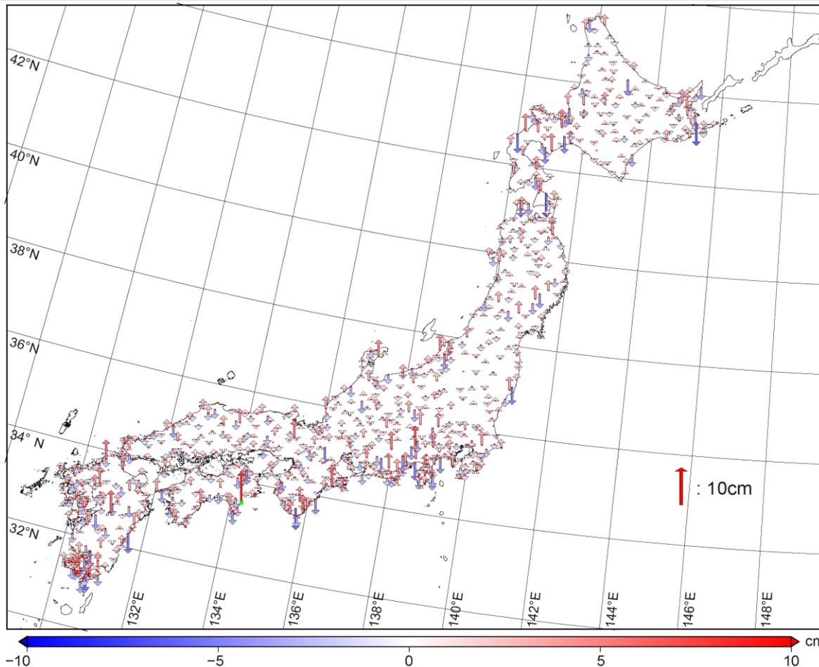
Reproduction errors (differences between GSIGEO2011 and GNSS/leveling).
