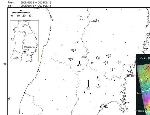
Coseismic vertical displacements at GEONET stations caused by the Iwate-Miyagi Nairiku Earthquake in 2008.
