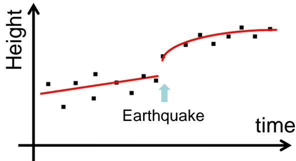
1. Modelling velocity at GEONET station by fitting coordinates to linear trend, coseismic displacement and postseismic movement (logarithmic function)
