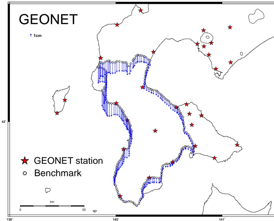
Vertical displacements on benchmarks from 2003-2004 to 2014 estimated from GEONET coordinate time series
