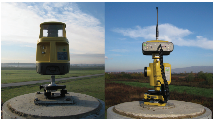
Figure 1 (a) PZL-1 laser transmitter and (b) PZS-1 sensor connected to GNSS rover receiver
