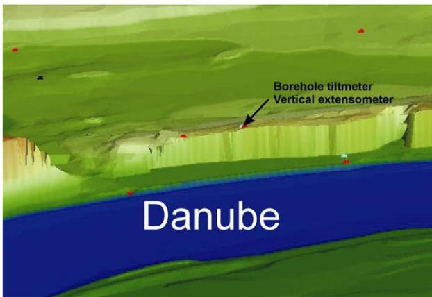
Figure 2. Digital Terrain Model (DTM) of the Dunaföldvár testsite. Red points denote the GPS monuments, blue points show the location of the tiltmeters
