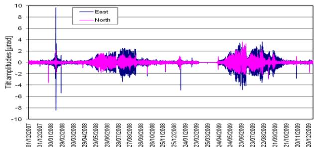
Figure 8. High-pass filtered tilt data measured at the Dunaszekcső test site from 1 December, 2007 till 31 December, 2009
