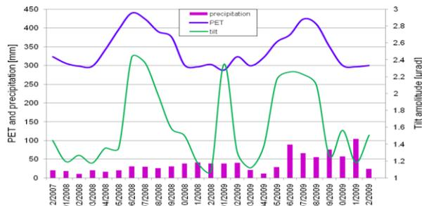
Figure 9. Relationships between PET, monthly averages of the precipitation and tilt amplitudes in the Dunaföldvár test site
