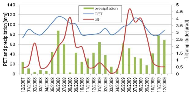
Figure 10. Relationships between PET, monthly averages of the precipitation and tilt amplitudes in the Dunaszekcső test site
