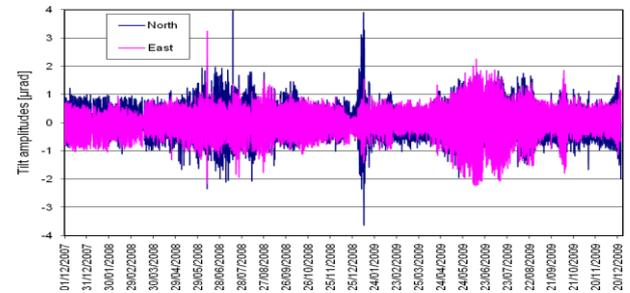
Figure 7. High-pass filtered tilt data measured at the Dunaföldvár test site from 1 December, 2007 till 31 December, 2009
