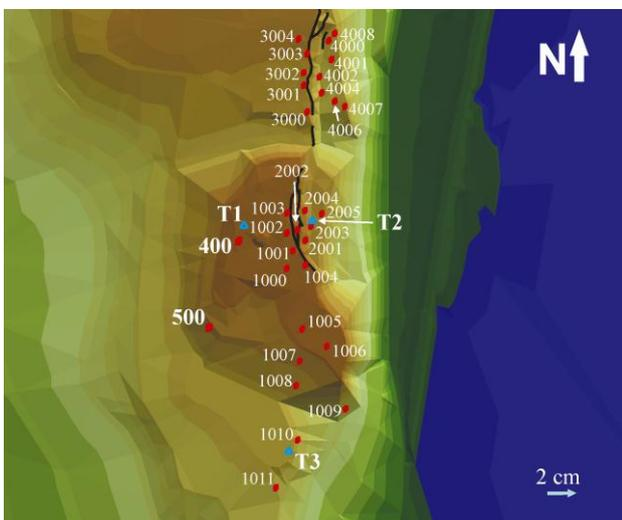
Figure 3. DTM of the Dunaszekcső test site with the location of tiltmeters (T1 –T3) and GPS monuments (red circles)
