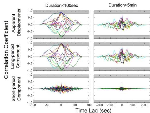
Figure 4. Typical cross correlation curves for two collocated Hiper Pro rover instruments. The gray-shaded area marks results with correlation coefficient  $> 0.8$ . No systematic evidence of a time lag between the two receivers exists. Results correspond with the vertical – Up Axis, while similar results were obtained for the horizontal Axes.
