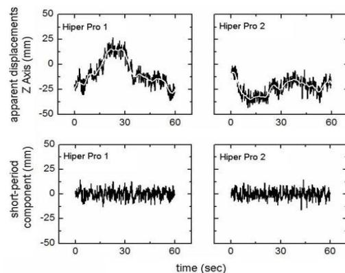
Figure 3. Apparent displacement time-series (upper row) from two collocated, simultaneously recording GPS instruments (noted as Hiper Pro 1 and Hiper Pro 2). The thick, white line represents the long-period component of the time series. In the bottom row the short –period component, resulting after subtracting the long-period component, is presented. It is obvious that each instrument presents a significantly different long-period component waveform.
